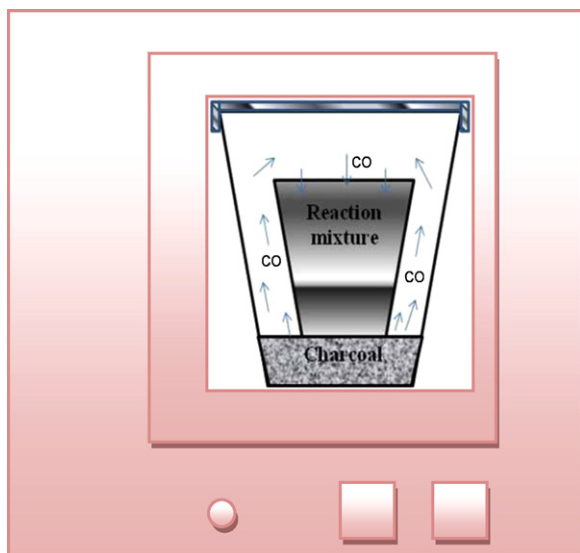
Fig. 1. Laboratory box furnace with two alumina crucibles. The smaller crucible contains the reaction mixture, and the larger crucible contains charcoal.
